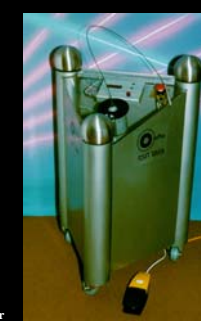
Fig. 11: Prototype of Tm:YAG and Er:YAG Laser
